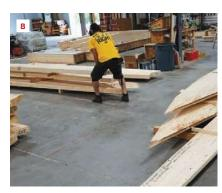
Alex Morin assembles the framing for a window rough opening. This component will then get fed into the automated framing system that will frame the other parts of the wall (3).
